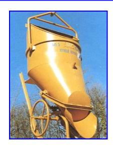
The skip is designed for the transporting and pouring of concrete in conjunction with a crane or other suitable lifting equipment. The crane must be of sufficient capacity to safely transport the combined weight of the skip and its concrete load. For estimating purposes the approximate weight of concrete (subject to mix) is 2400kgs per cubic metre.
