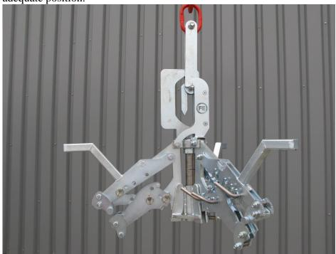
**Lifting manhole bases.** Loose the locking pin and strike the cone valve upwards. Lock the
