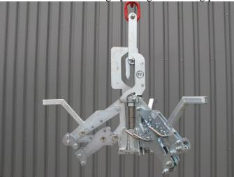
**Lifting DIN 800 mm shaft parts.** Loose both locking pins and shift the conce valve forwards. Lock the cone valve by using the locking pins.
