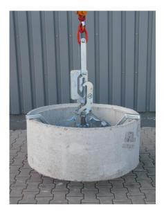
All circulation pipes need to rest on the upper edge of the manhole ring Put the hanger in the circuit board in position "hoist cone". Then hoist slowly and evenly
