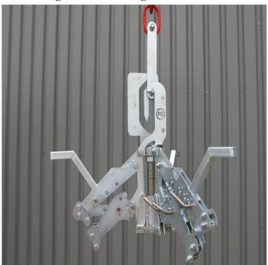
Lower the manhole lifter in loosened position in the manhole ring to be lifted
